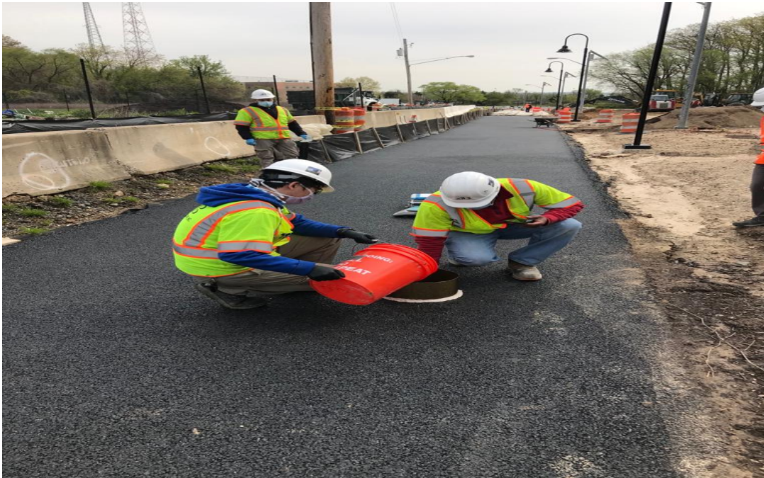
Phase B – QA Inspectors performing infiltration test on the new trail
