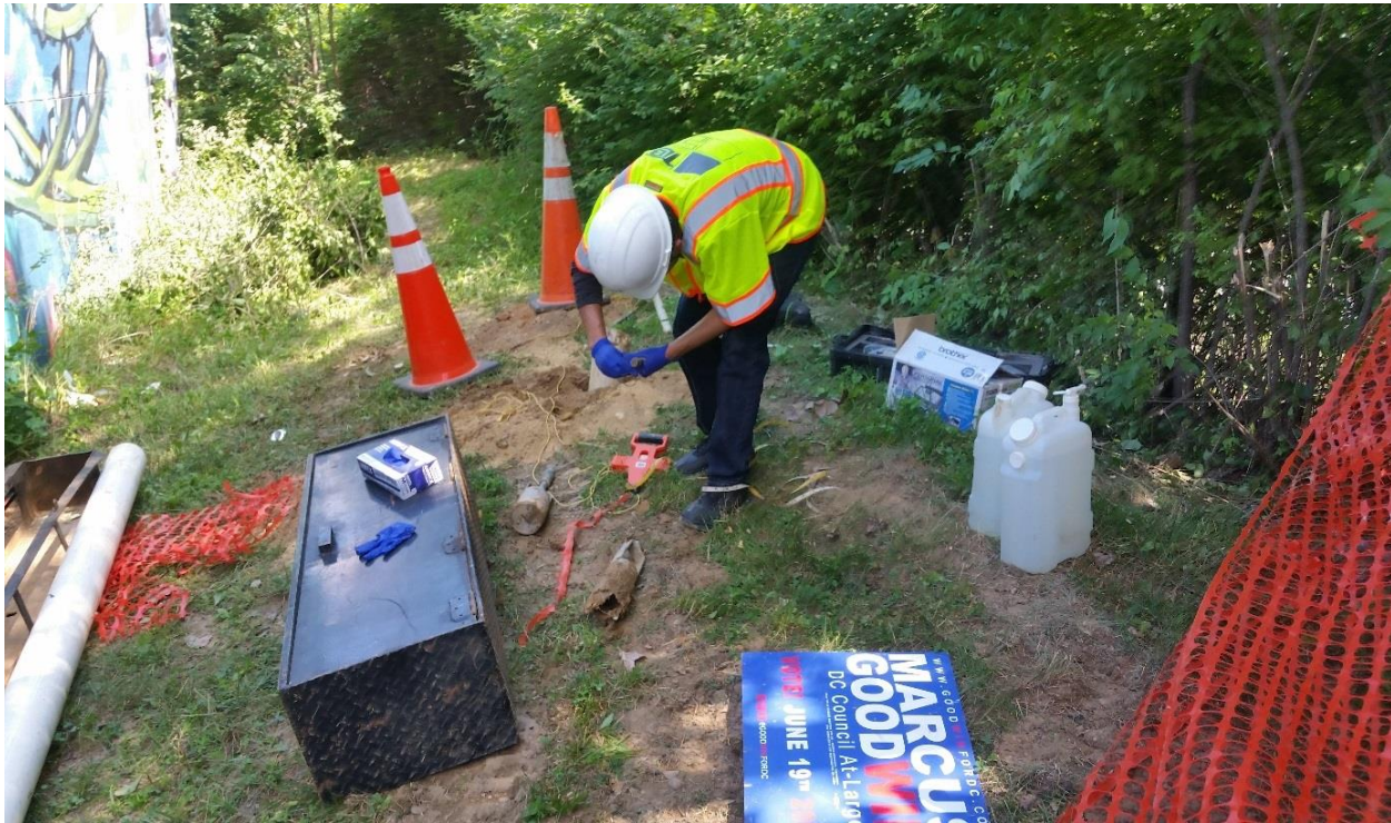
Performing an Infiltration Test (Phase D) near the intersection of Bates Road and John McCormack Drive
