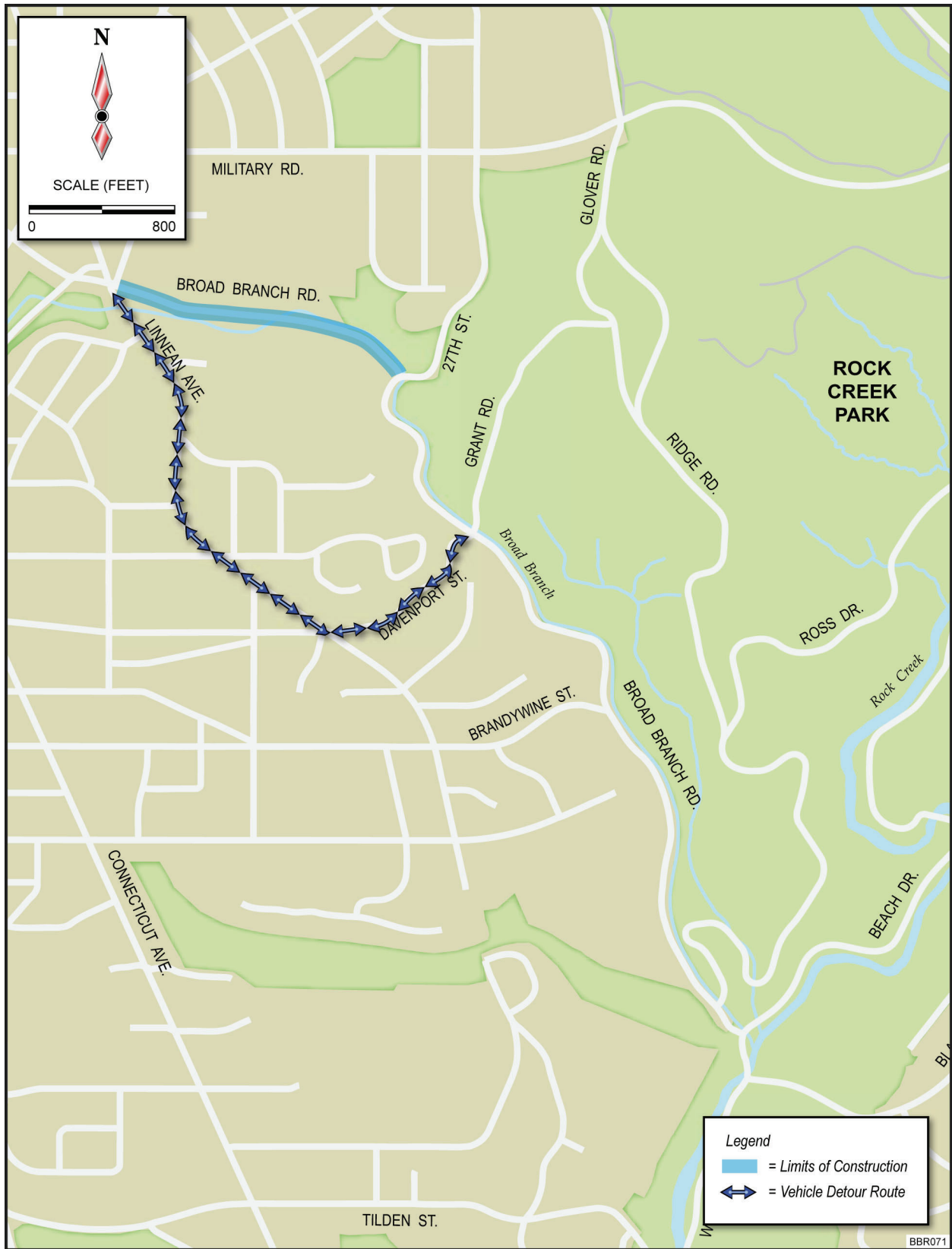
Figure E-1. Potential Detour – Location 1
