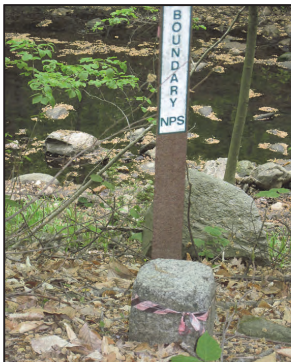
Figure 3-8. Modern Metal Witness Post co-located with the older stone boundary marker
