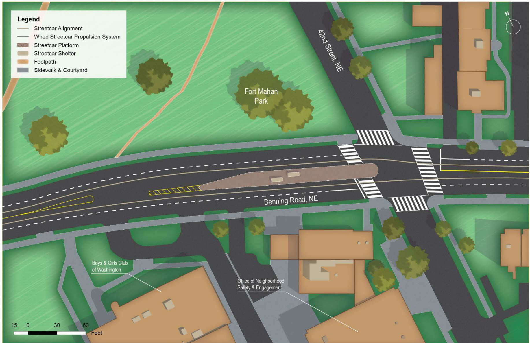
Figure 4-2: Conceptual Drawing of 42 nd St Streetcar Stop and Roadway Configuration
